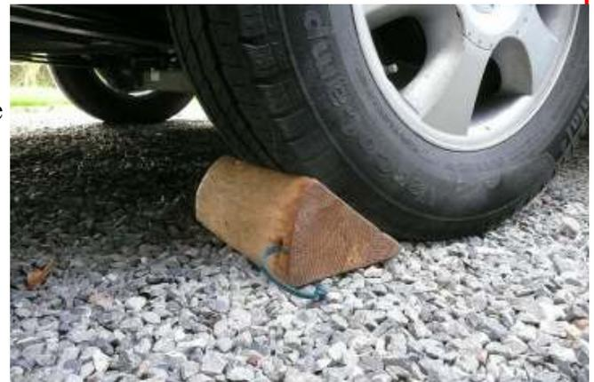
The picture on the left shows one of the finished chocks. I included a loop of rope so that they can be pulled out easily.
