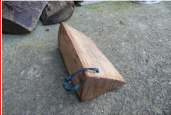
Well the problem with leaving it up on chocks is that you need to make sure it does not run down the chocks hence one puts the hand brake on. The problem I have encountered in the past is..... sticking / binding
